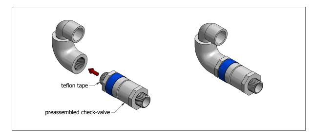
Step 18: Attach elbow to other end of check valve.
