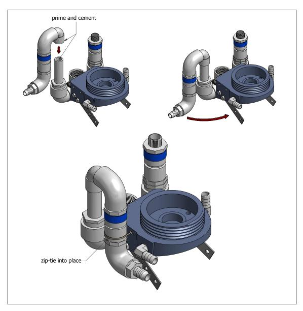
**Step 20:** Attach elbow of previous assembly to pipe piece.
