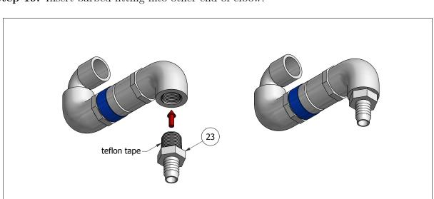
**Step 19:** Insert barbed fitting into other end of elbow.
