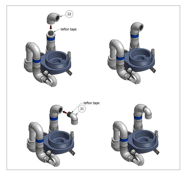
Step 22: Attach full male thread elbow and male thread, female socket elbow.
