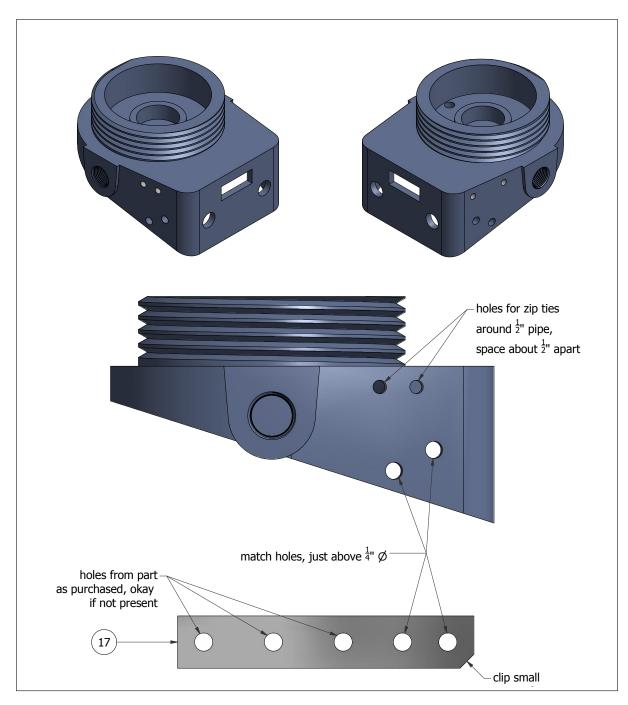
Step 13: Drill matching holes in filter bowl head and though metal strips.
