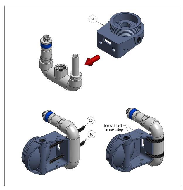
Step 12: Attach filter bowl head to previous assembly with hose clamps.
