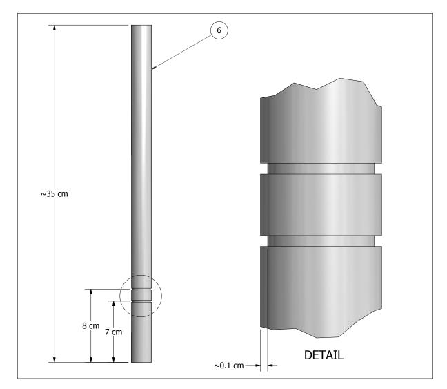
**Step 05:** Cut two recesses in exterior surface of 1/2" pipe piece.
