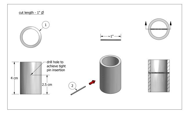
Step 01: Drill holes in pipe piece and insert nail.
