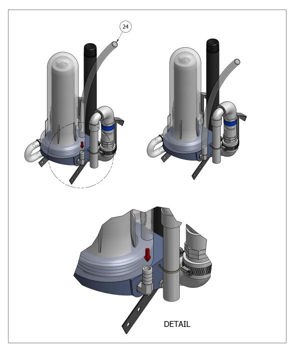
Step 27: Attach inlet tube and secure with hose clamp.
