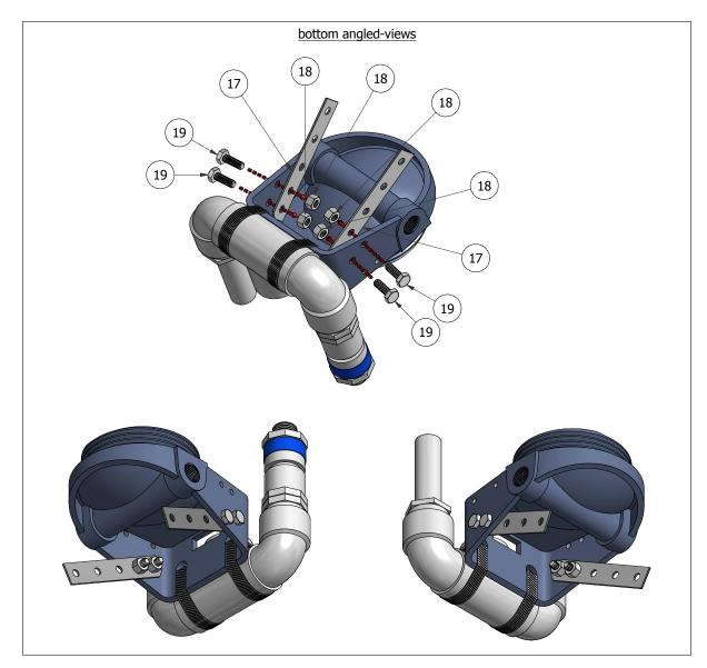
Step 14: Attach metal strips to filter bowl head.
