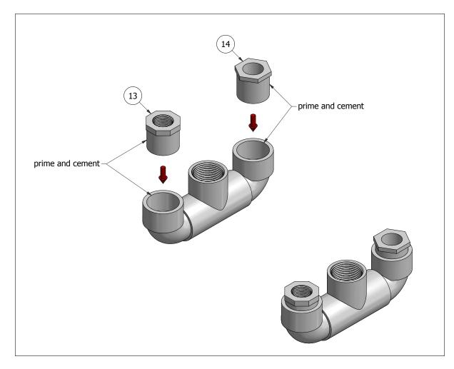
Step 09: Cement in place a socket bushing in one elbow and a threaded in the other.
