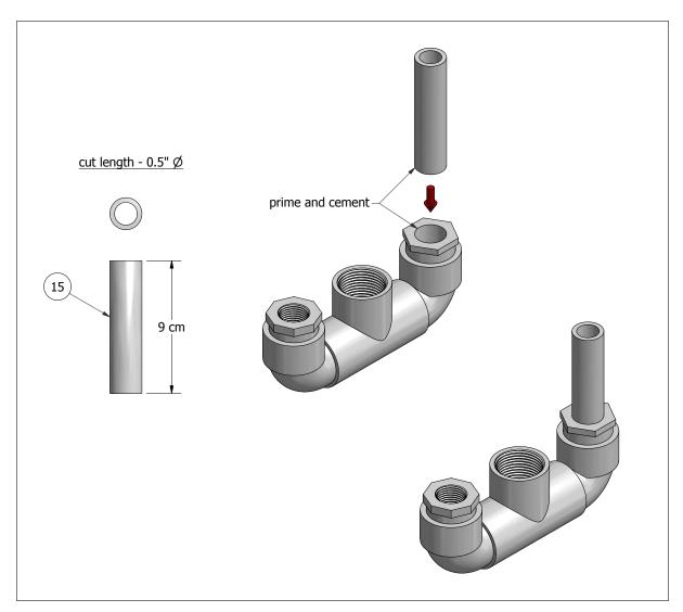
Step 10: Insert a pipe piece into the socket bushing and cement in place.
