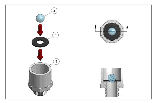
Step 02: Drop rubber washer and marble into a reducer.
