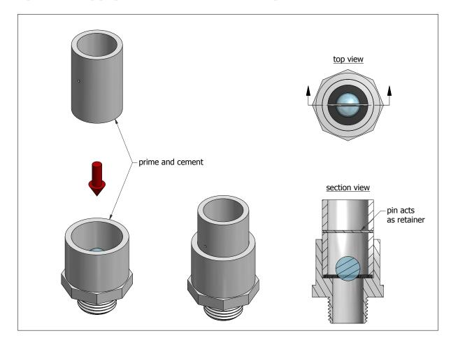
Step 03: Insert pipe piece into reducer and cement in place.
