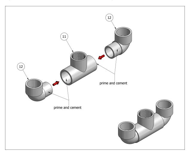
**Step 08:** Insert two elbows into a tee and cement in place.
