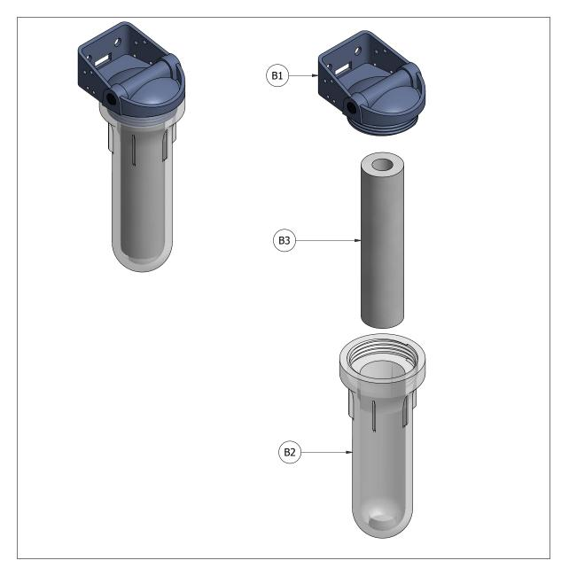
${\bf Step} \ {\bf 07:} \ {\bf Separate \ parts \ of \ filter \ bowl.}$
