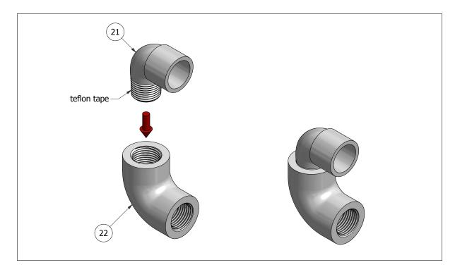
Step 16: Insert male thread, female socket elbow into full male thread elbow.
