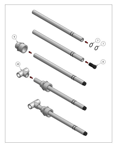
Step 06: Slide 2 O-rings onto pipe, insert plug, attach adapter and tee.
