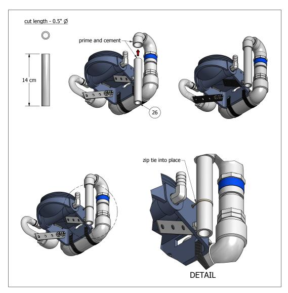
Step 23: Insert pipe piece into elbow and secure with zip tie.
