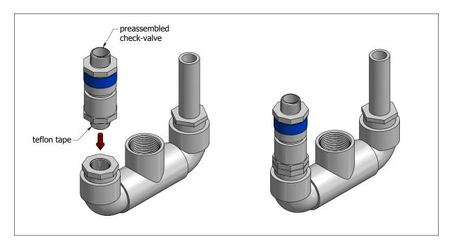
Step 11: Insert one of the check valves into the threaded bushing.
